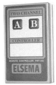
The battery service life approximates its shelf life. 9-Volt Carbon or Alkaline type batteries may be used. Depending on the battery type, shelf life ranges between 1 and 2 years. While the FMT-202 is not transmitting it uses no power. It will operate on as low a 4 Volts DC, however, in such cases the power and range will be reduced.
